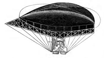
A fan or propeller is driven by treadle mechanism, and the passengers are provided with seats within a closed car. Four boats are carried below the car for supporting the apparatus should a descent be made on water. A.D. 1889.
